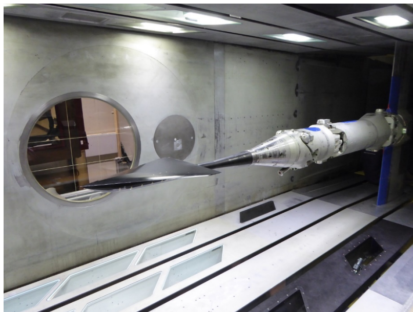
Figure 2: WEAG model in the DNW-HST slotted test section
